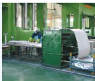
② Raw material sheet cutting
