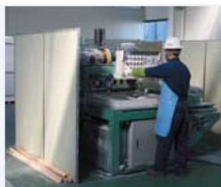
⑥ Trimming and making hole
